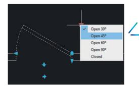
Dynamic Blocks can be inserted and displayed, which makes it more convenient for you to modify the blocks simply by clicking the grips.
