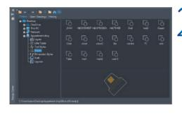
It allows you to search and access any CAD resources stored in your computer or other computers on your local network. You can insert layers, line types, text styles, blocks, etc. from other drawings to the current, enabling you to design with more resources.
